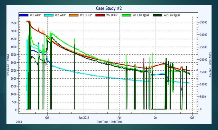
Wellhead and downhole pressures and individual calculated rates
