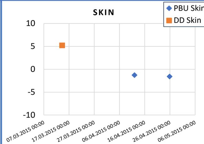
Each PBU and DD test are analyzed for diagnostic PTA parameters in real-time
