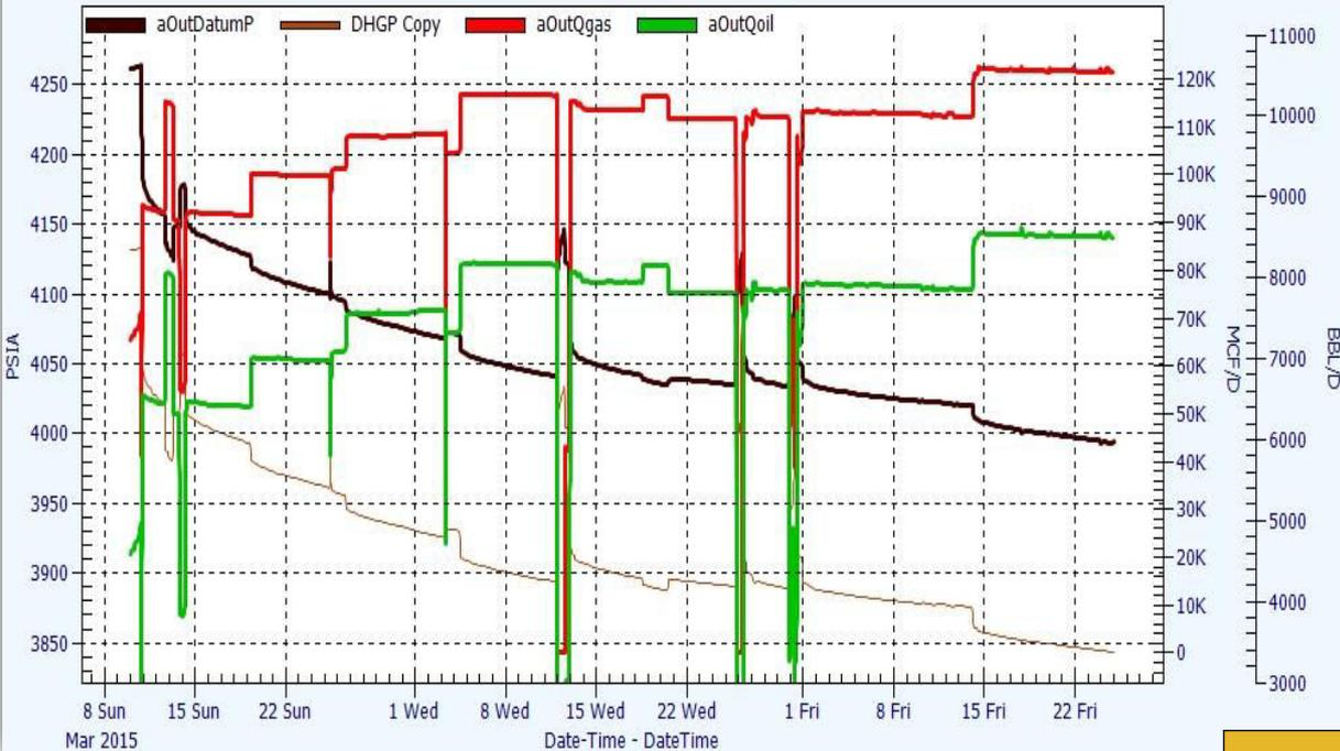
The tool calculates **multiphase rates** using dP in the wellbore using a **direct numerical integration** to the Mechanical Energy Balance and **rigorous PVT**
