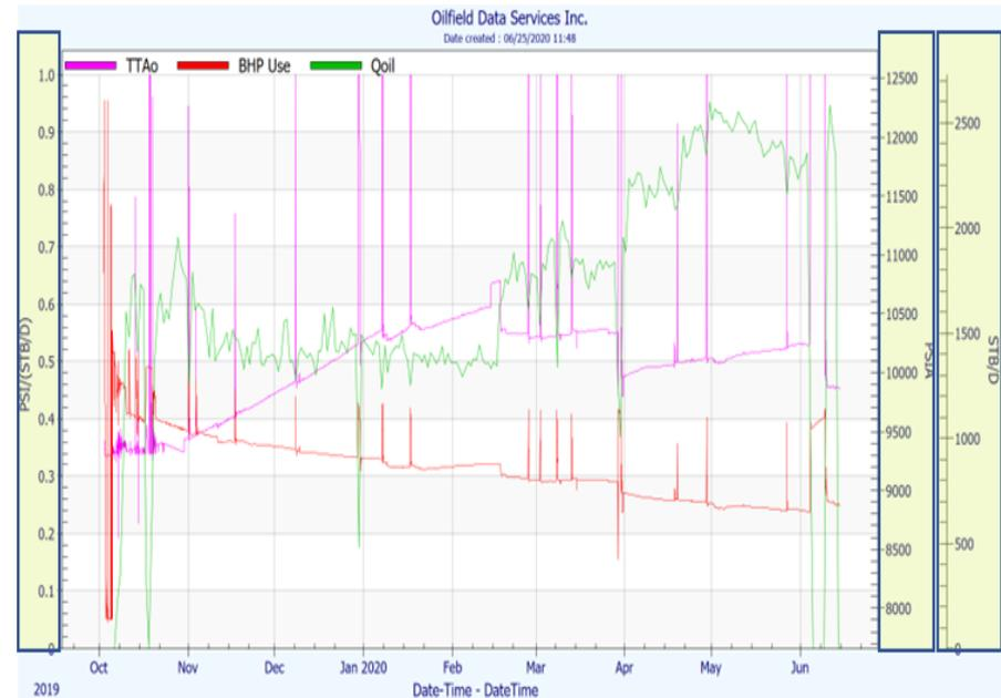
The analysis is used to determine Hydraulically Connected and Mobile HC volumes and how they are changing with time.
