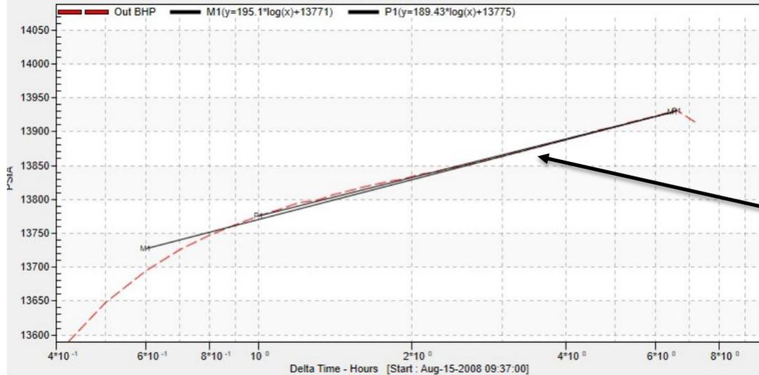
m-slope is selected at the same time as the radial flow period in the derivative plot
