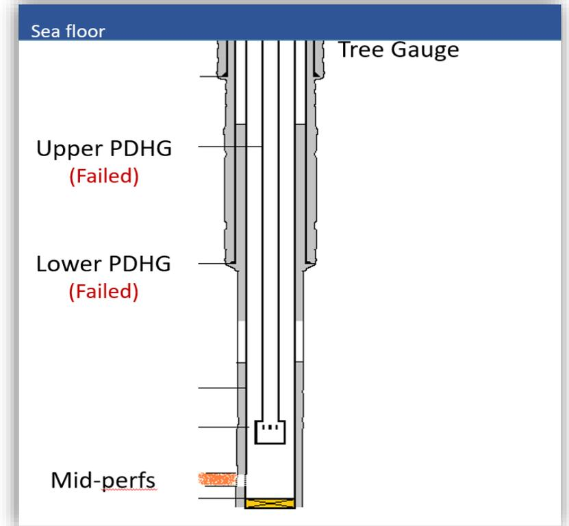
All PDHGs failed. The interpretation was done on the historical data with functional gauges to demonstrate the accuracy of ODSI's BHP conversion and to demonstrate that the well was not a stimulation candidate
