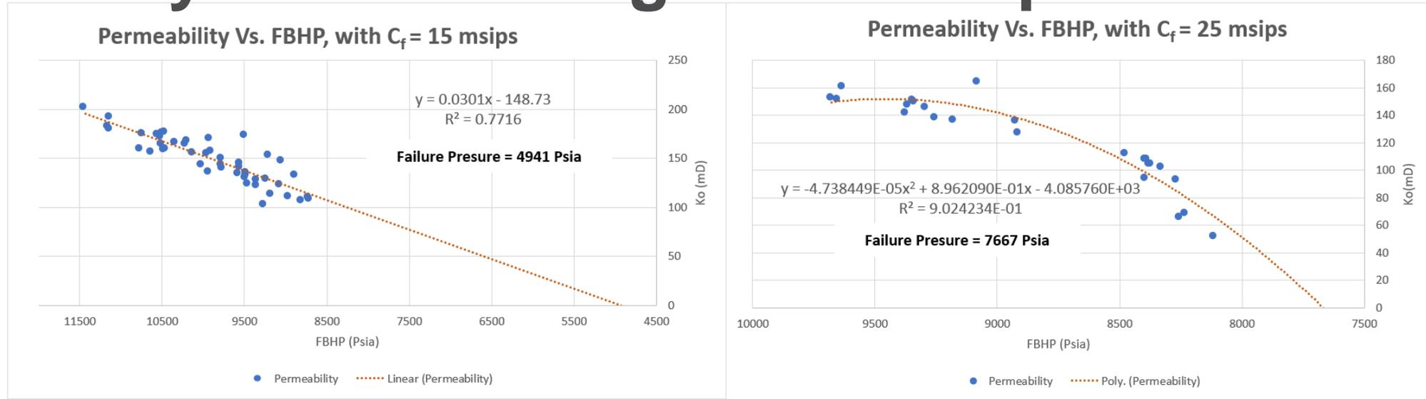
Figure 6 – Impact of the permeability curve and flowing bottomhole pressure on shear failure prediction
