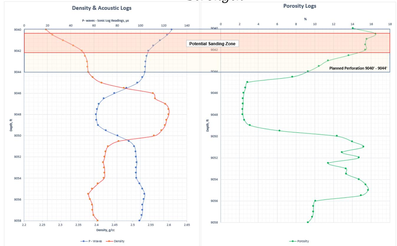
Figure 5 – Density/acoustic and porosity logs for the same formation as Figure 4. Note the orange box indicating a potential sanding zone in the upper planned perforation zone.
